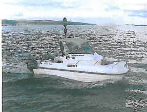
Below: 5m trailerable NoosaCat Felix using an interferometric wide swath survey system located in a centre aft position between the engines
