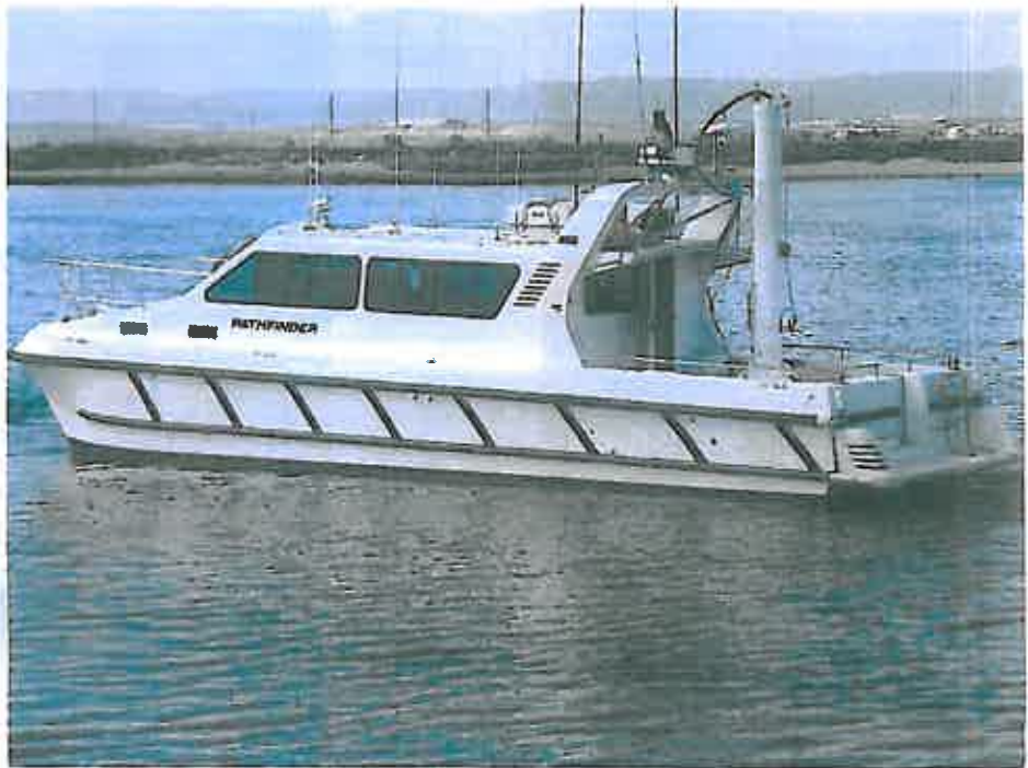
Above: 11m NoosaCat Pathfinder using an interferometric wide swath survey system mounted in a moon pool between the hulls
