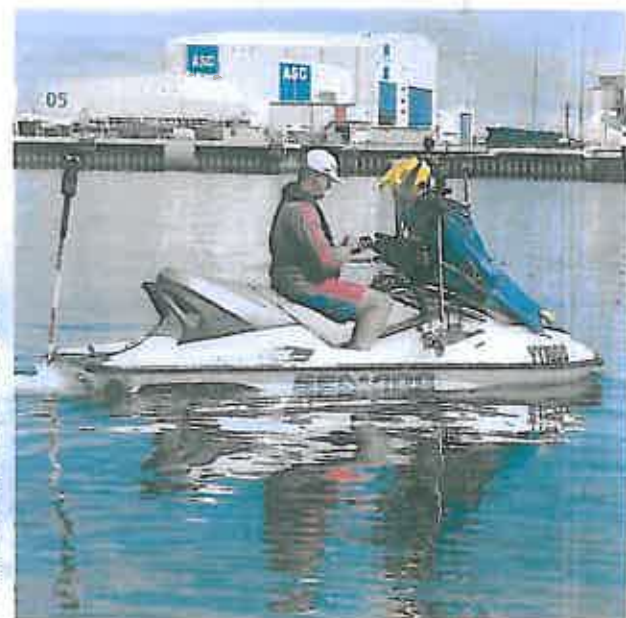
Below: Fully customised SeaDoo JetSki using a single beam echo sounder
